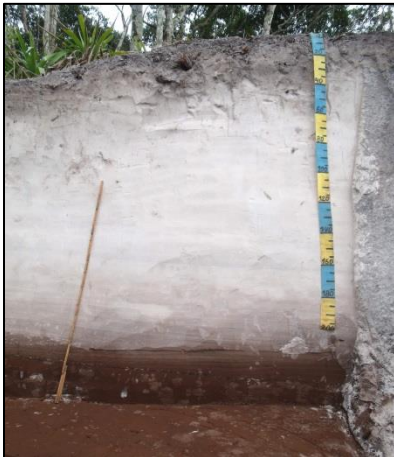
Fig. 4a. Stop 2 (profile PF01): Podzol that originally formed under poorly drained conditions; cliff formation then improved drainage.
