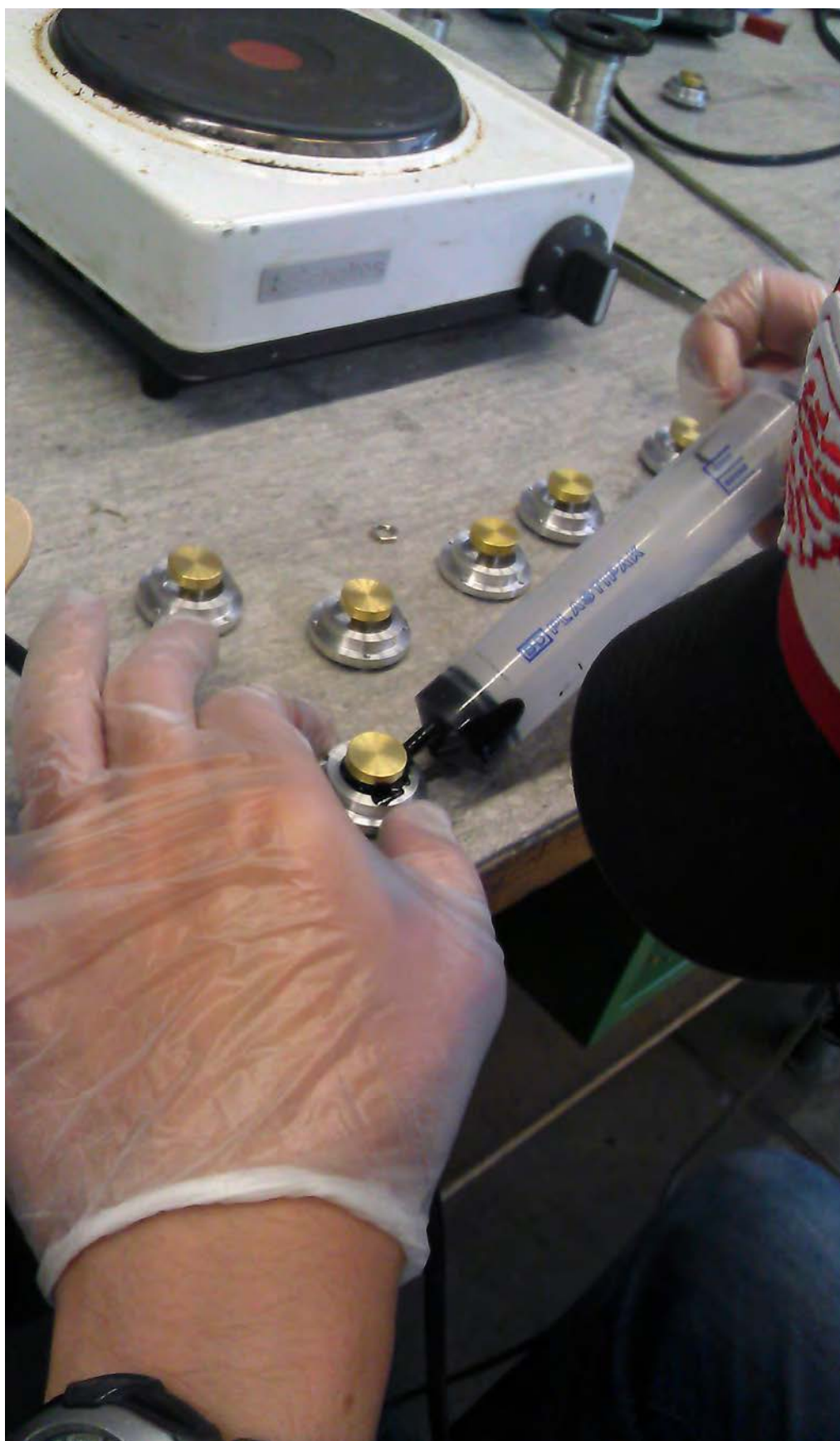
Figure 9.8.: Picture of the injection of the liquid glue under the electrode.
