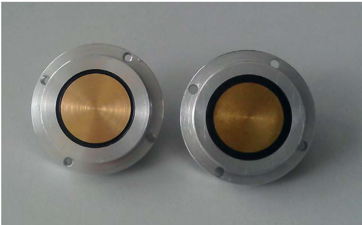
Figure 9.12.: Picture of two OST electrodes in their casings, on the left a CERN built one, on the right the version from Cornell University.
