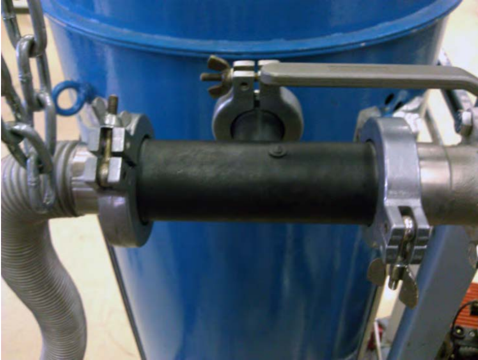
Figure 9.5.: Picture of the insulating element in the metal pump line.
