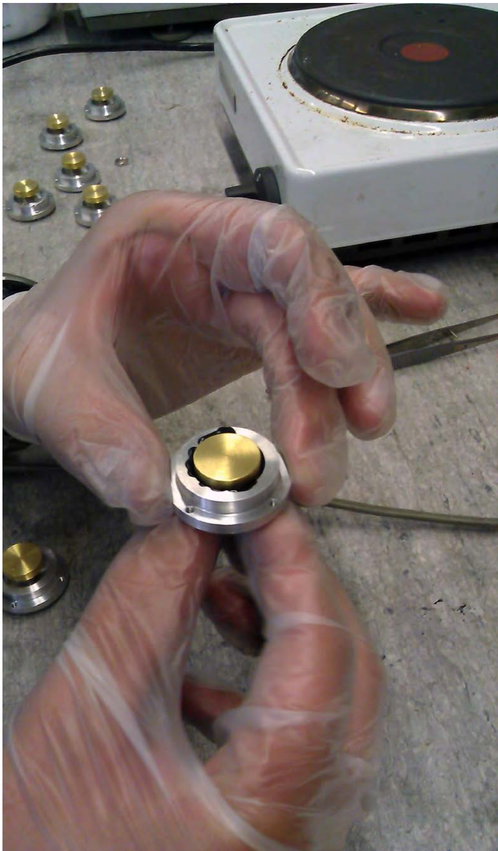
Figure 9.9.: Picture of the glue spreading process via lowering the electrode in the casing.
