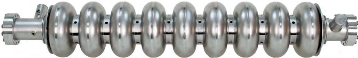
Figure 1.2.: A TESLA cavity made out of pure Niobium, from [1].
