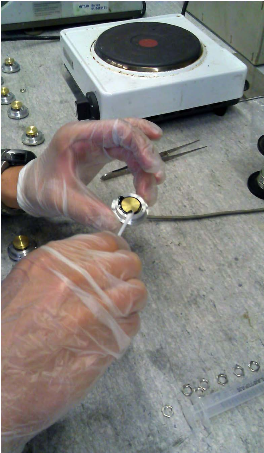
Figure 9.10.: Picture of the final cleaning of the back part of the OSTs casing.
