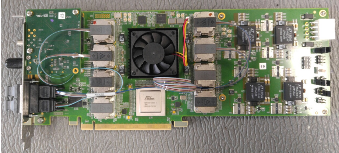
Figure 2.10.: An image of the FLX-712 custom FELIX hardware. Half of the miniPOD fibre optic transceivers are used, corresponding to the 24 of the maximum 48 available links. On the front panel, one MTP24 connector per FELIX device is exposed to the user.
