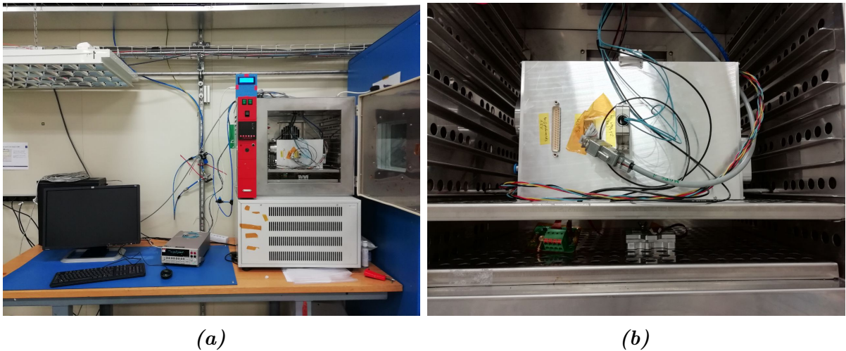
Figure 6.6: Experimental setup of the climate chamber measurements of the optobox, module and interlock NTC in SR1 (a) with a closer look inside the climate chamber (b).
