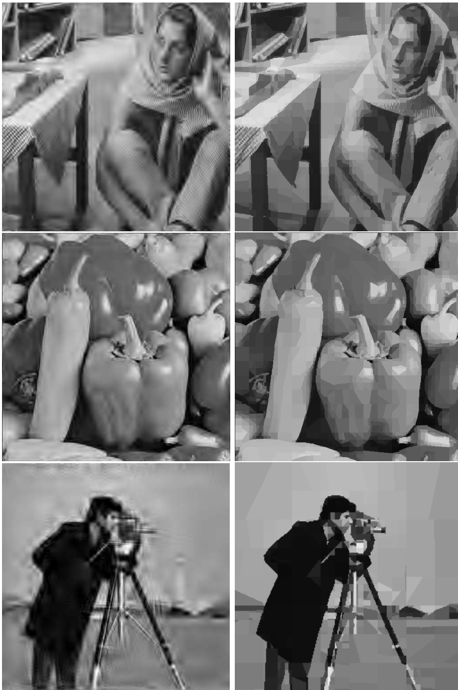
Figure 1.12: Sample reconstructions using 0.01 coefficients per pixel, for contourlets (left) and wedgelets (right). Top row: Barbara, with contourlets: 23.89 db, wedgelets: 23.02 db; middle row: Peppers, with contourlets: 28.12, wedgelets: 27.84 db; bottom row: Cameraman, with contourlets: 22.90 db, wedgelets: 23.82 db
